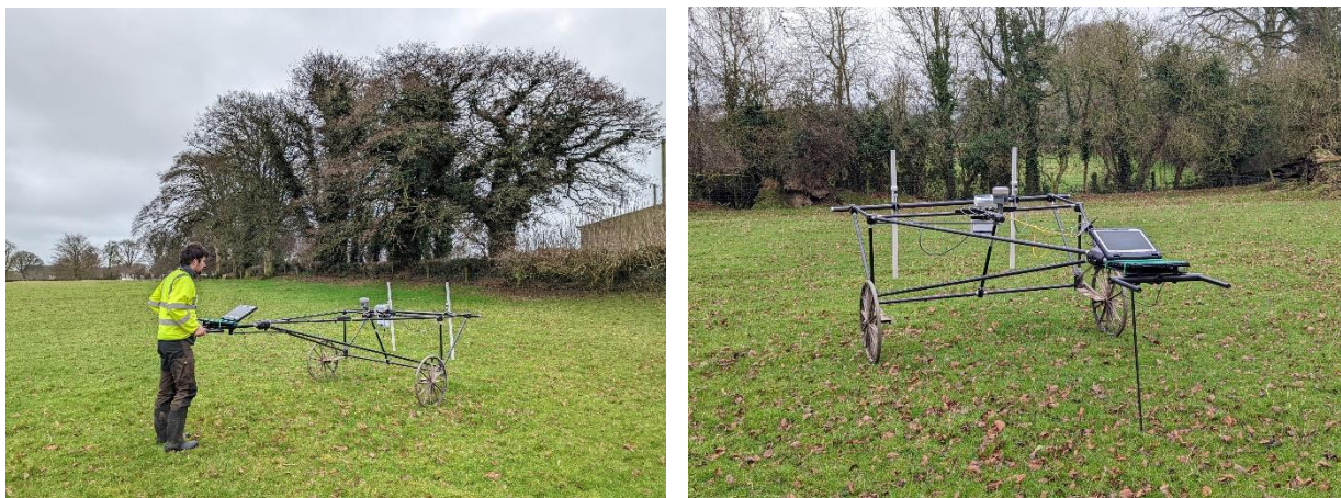
Bartington Grad 601-2 mounted on Bartington Cart system
